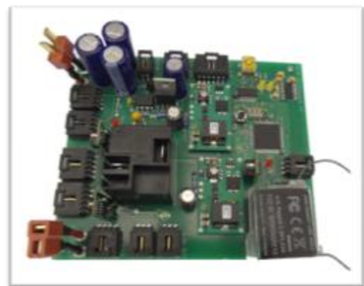
Figure 3: MOLLEBot's Custom Power and Control Board
